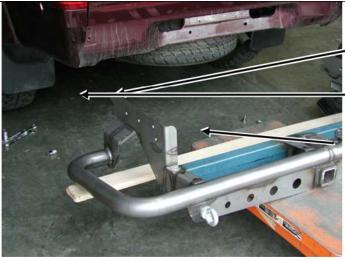
7. Guide the new rear step under the vehicle and onto the protruding M12 bolts already in position. Take care not to damage the vehicle panels.
