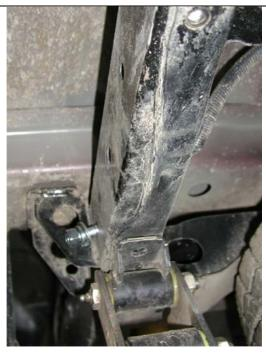
6. Fit the M12 x 1.75 X 40 long hex bolts, flat washers, spring washers and nuts through the holes in the chassis (closest to the suspension bracket as shown) on both sides of the chassis. (2 bolts, 4 flat washers, 2 spring washers & 2 nuts)
